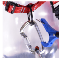
Step 4 Hook the carabiner onto the harness fall arrest point and pull rescue pole back to release.
